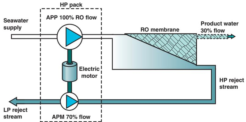
APM—axial piston motor, APP—axial piston pump, HP—high pressure, LP—low pressure, RO—reverse osmosis
