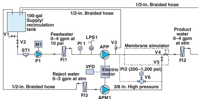
APM—axial piston motor, APP—axial piston pump, EM—electric motor, FI—flow indicator, LPS—low-pressure switch, PI—pressure indicator, VFD—variable-frequency drive, V—valve
