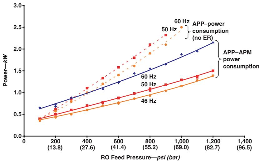
APM—axial piston motor, APP—axial piston pump, ER—energy recovery
