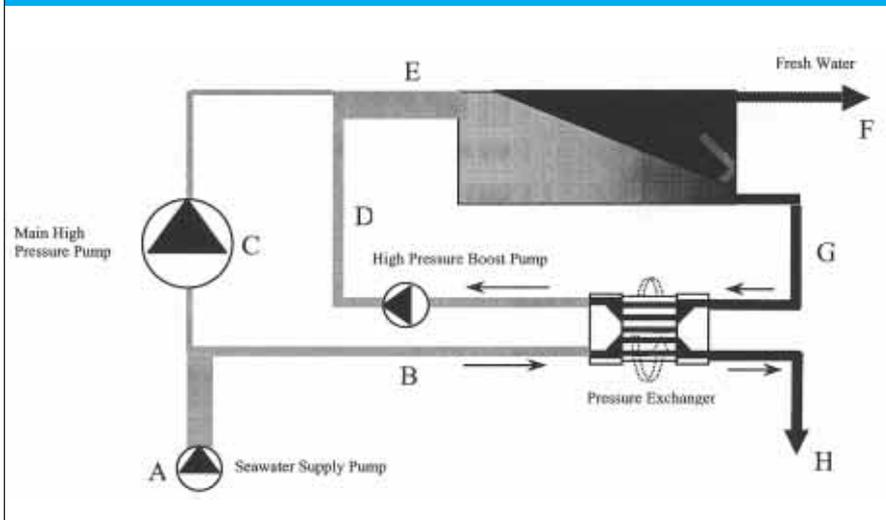
Since the PX unit is providing nearly 100% of the reject flow at 95% efficiency, there is very little energy penalty for increasing this flow and thereby lowering the recovery rate of the RO system. At lower recovery the pressure required to produce the same amount of product water is lower, resulting in lower power consumption.
