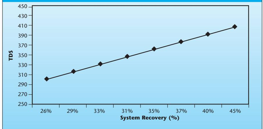
small impact on overall capital costs. For example, decreasing the recovery of a 1000 m<sup>3</sup>/day system from 45% down to 35% will increase the membrane feed flow from about 400 gpm to 520 gpm. This would typically require 4in (100mm) PVC pipe in either case.
