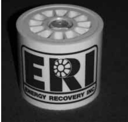
By rotation the ducts are first exposed to low-pressure feed water, which fills the duct and displaces the reject water. The rotor continues to rotate past the sealing area and is then exposed to the high-pressure concentrate, which fills the duct and displaces the feed water at high pressure. This rotational action is similar to a Gatling gun firing high-pressure bullets and being refilled with new seawater cartridges. Figure 1 below depicts a sectional view of these dynamics.
