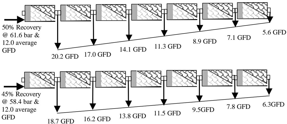
Decreasing the system conversion and flux rates does have its disadvantages, mainly by increasing the size of the pretreatment system and membrane stacks. This effect is less significant in smaller systems under 1000 m<sup>3</sup>/day because of the less expensive piping materials, pressure media filtration systems and
