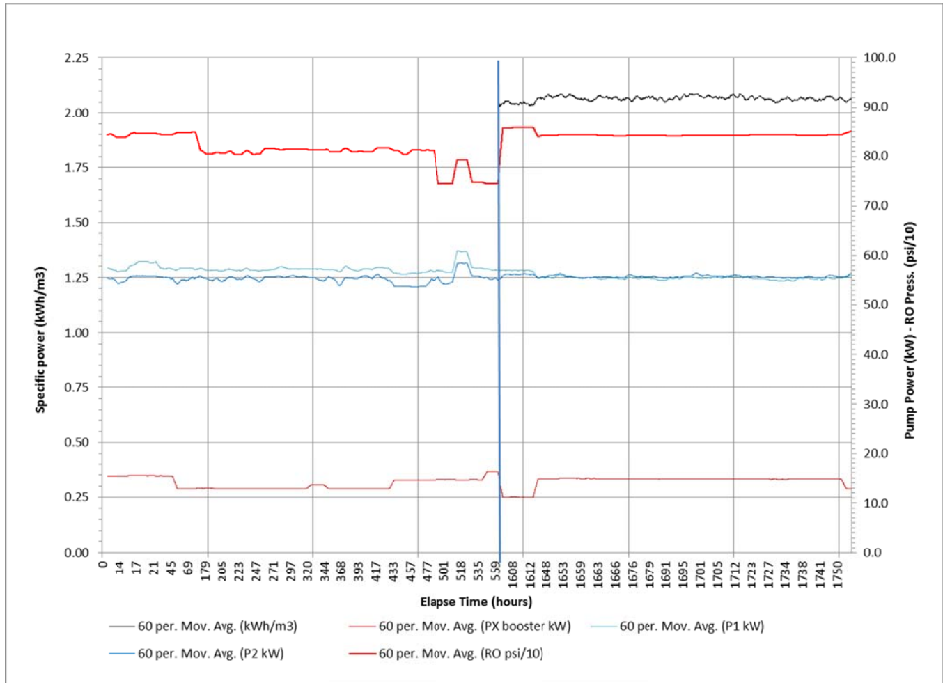
Figure 7. Power and RO Feed Pressure Over Time
