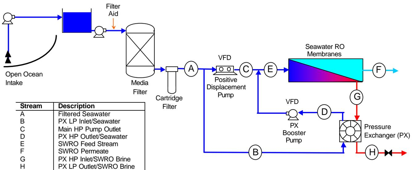
**Figure 1. Process Flow Diagram - ADC's Demonstration Scale SWRO plant**
