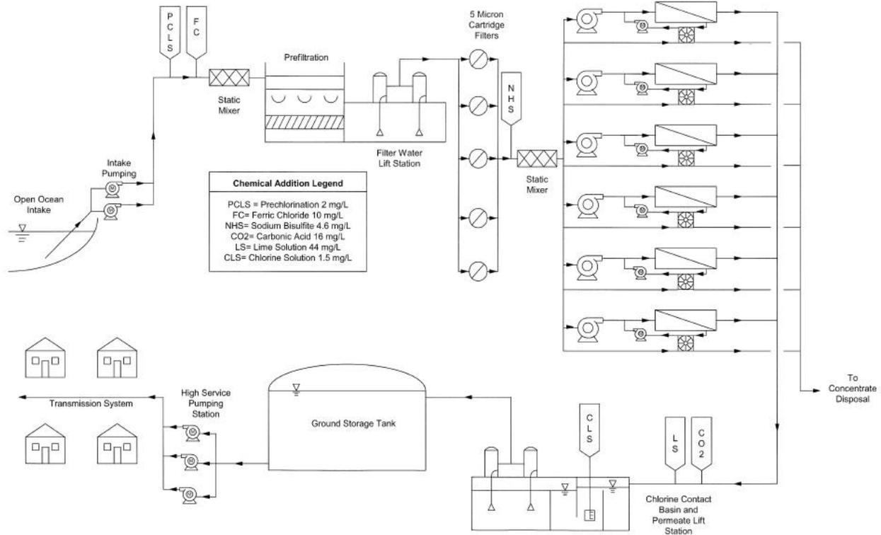
**Figure 3. Conceptual 10 MGD SWRO facility (Dedicated Pump Design)**
