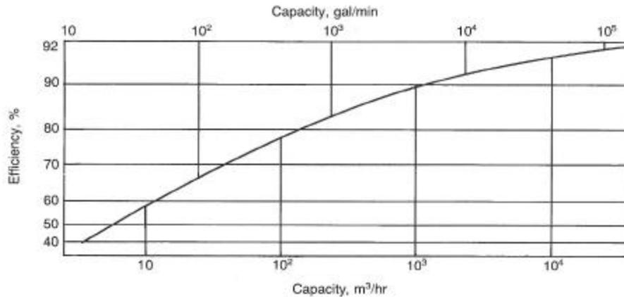
**Figure 2. Maximum Pump Efficiency Attainable at the Best Operating Point <sup>3</sup>**
